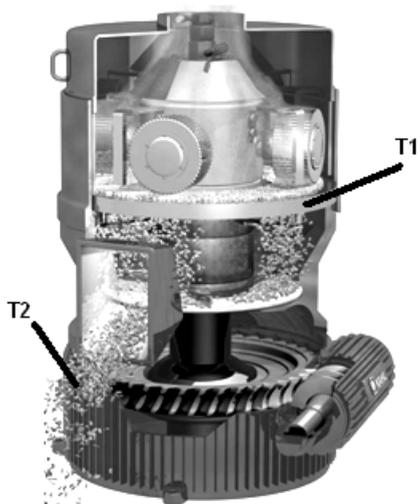
Figure 1 Flat die pellet press.
