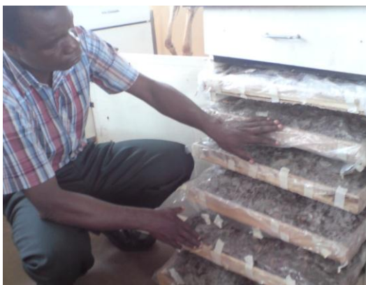
Figure 2: Fermentation chamber with six trays drawn out to show the arrangement of trays within the chamber.
